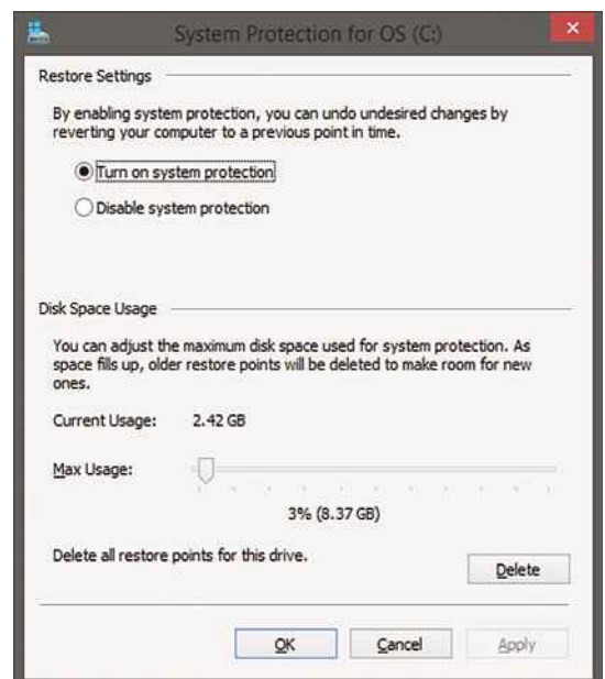
▲ If HDD space is a problem, you can disable System Restore or limit the amount it can use
