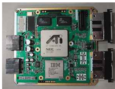
▲ The motherboard of the GC, with the Flipper GPU
