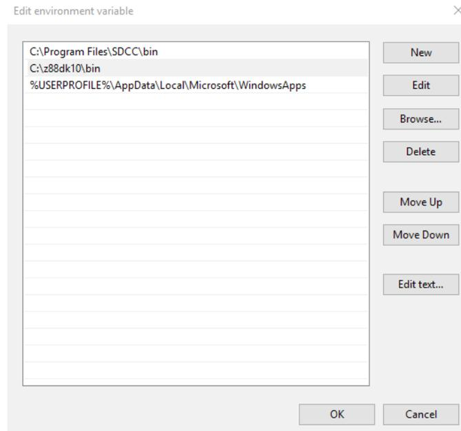
As you should see from my screenshot, SDCC and Z88DK are already entered. On your machine, SDCC should already be added to the path when you installed it, if not, then you are going to want to install it.
