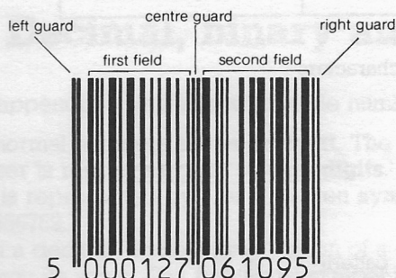
Fig. A3.1 The coding divisions for an EAN13 product code
