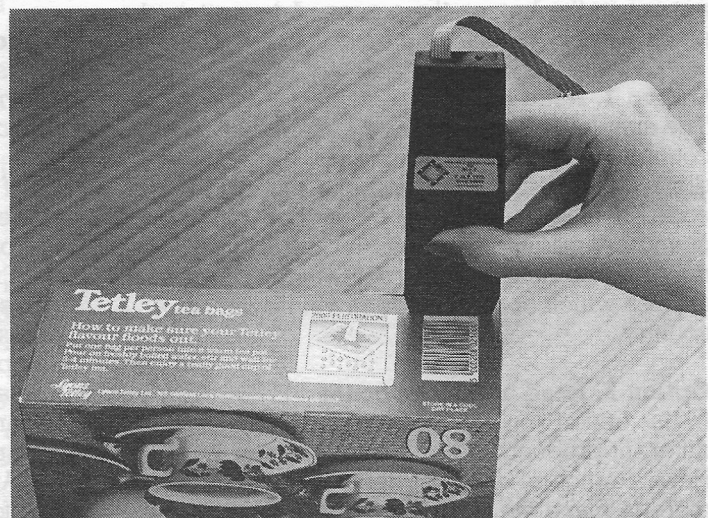
Fig. 6.1 The EAN13 product code being scanned
